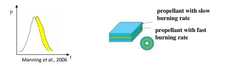
Manufacturing and characterization of type ABA propellant grains
